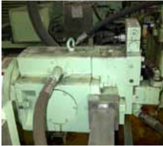
Eaton's PVX heavy-duty high pressure pump provides ample power supply for a 210-gpm/5,200-psi hydraulic power source.
