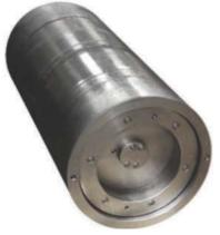
Patent-pending Lockbox piston accumulator design does away with threaded retaining rings to secure the end cap. This makes servicing faster and less complicated because it can be performed on-site using standard tools.
