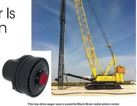
to control speed and torque. The motor has a hollow shaft, so grout, concrete, or other material can be pumped right into the center of the hollow auger.
